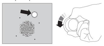
Taking care to protect your fingers in case the bulb should shatter, unscrew the old bulb.
